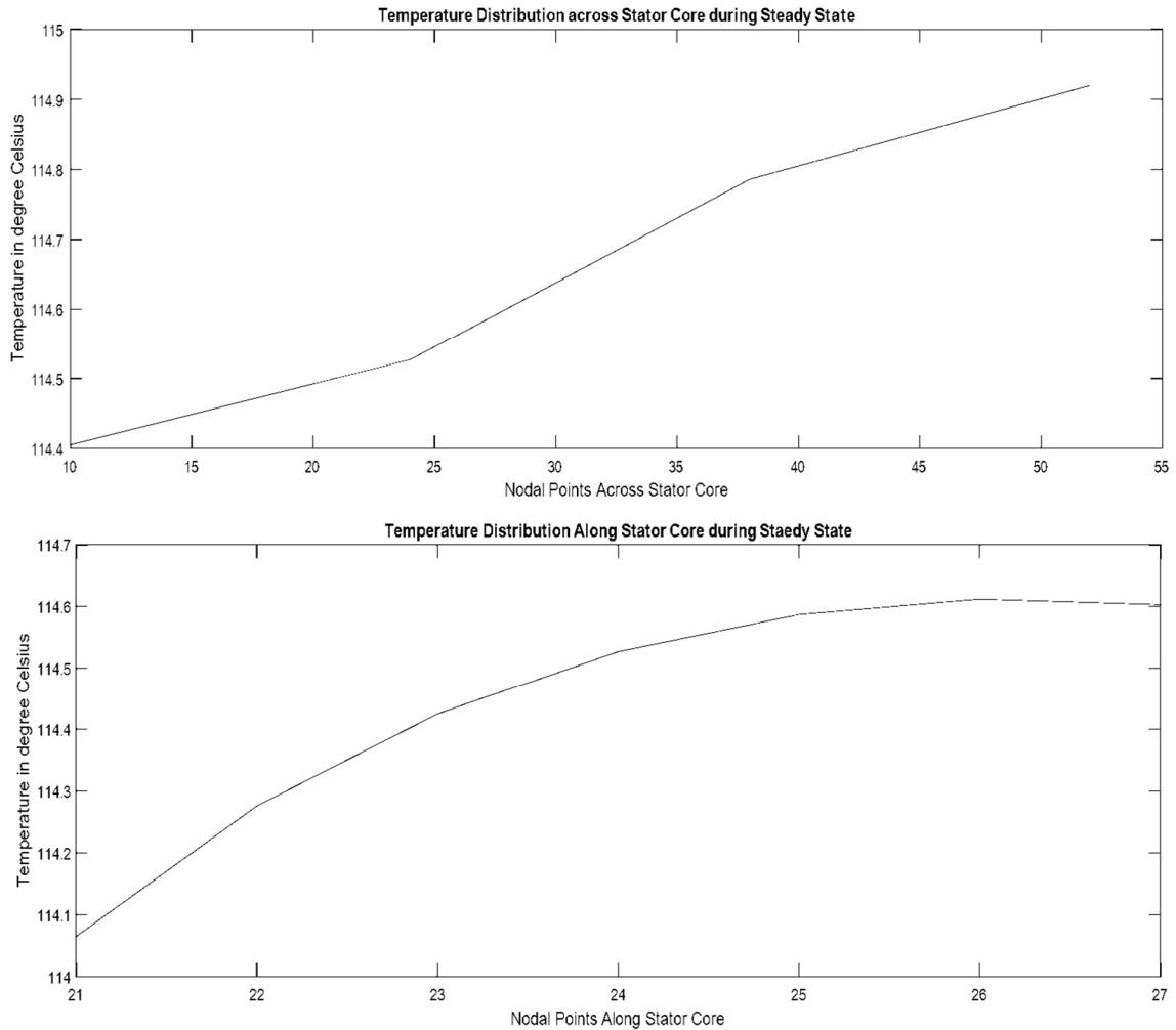
Fig 6:-Temperature Distribution across and along Stator Core
