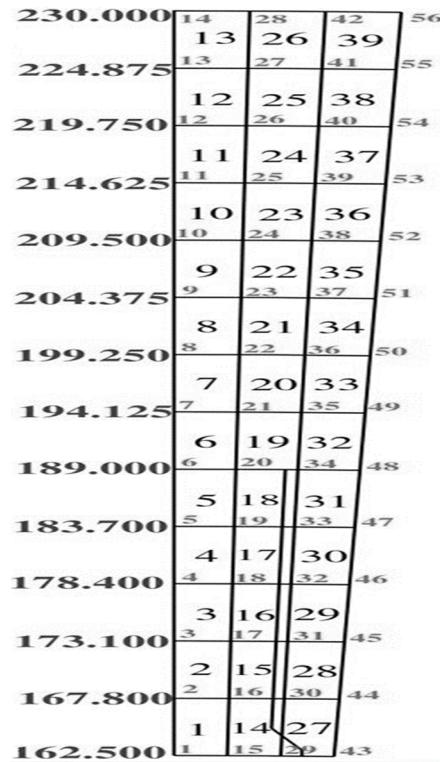
Fig. 3. Slice of core iron and winding of stator of slip ring induction motor bounded by planes at mid-slot and mid-tooth divided into arch shaped elements
