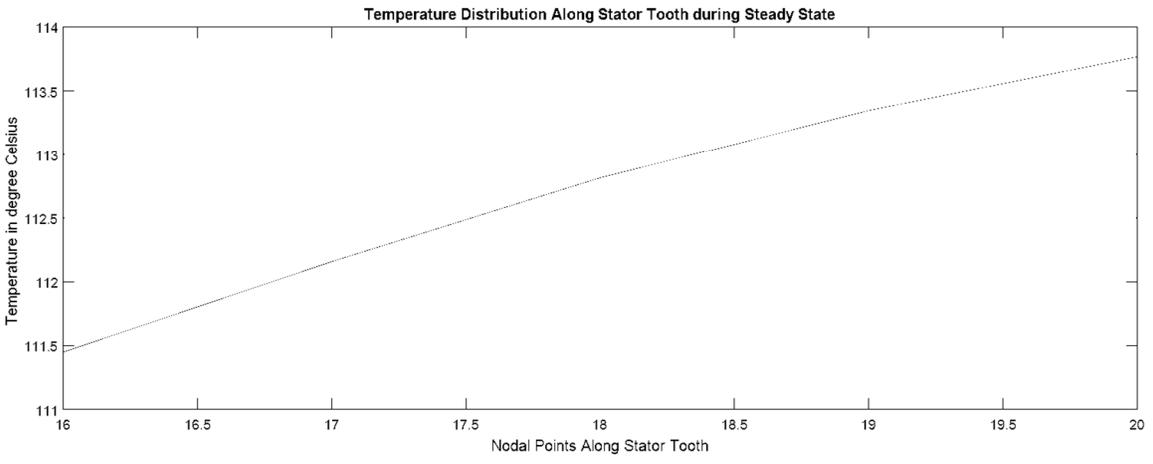
Fig 5:-Temperature Distribution across and along Stator Tooth
