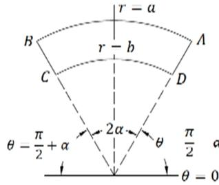
Fig. 1. 2D Arched shaped element suitable for discretization of induction motor stator
